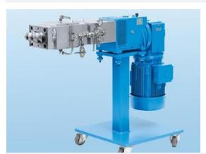
The ZS-B twin screw side feeder for ZSK extruders enables the side feeding of fillers and additives in powder or pellet form or cut glass fibers into the processing section of the twin screw extruder. The ZS-B features a self-cleaning profile of the twin screws and product feeding into the screw flights of the extruder without stagnant zones. Very little space is required for the side feeder thanks to its compact design.
