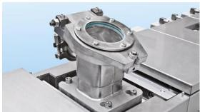
The feed hopper for ZSK extruders is only clamped to the process section with bolts. It can be removed very quickly by simply loosening these bolts. Then the quick-release insert which protects the barrel wall from contamination can very easily be changed.
