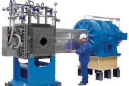
Use of a melt pump is necessary in individual cases for processing and pelletizing polyolefins. It ensures the necessary pressure build-up for the melt filtration and pelletizing at a very low introduction of energy. The Melt Pumps MP from Coperion are adapted individually to the project requirements as well as the ZSK MEGAcompounder.
