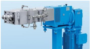
In this patented technology the feeding zone of ZSK extruders is equipped with a porous, gaspermeable wall section to which a vacuum is applied externally. The resulting gas extraction increases the material intake capacity in the processing of feed limited products by up to three times.
