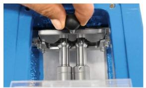
For ZSK 26 Mc<sup>18</sup> laboratory extruders Coperion has developed a patented quick-release screw shaft coupling that enables screw changes to be performed as quickly as possible. Cleaning times are reduced to a minimum when changing colors and recipes.
