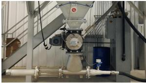
The specially designed high pressure Coperion ZVH rotary valve is used for continuous gentle conveying of coarse granular or pellet size, friable or temperature sensitive materials such as plastic pellets, coffee beans, grains, etc.
