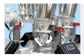
The K4G system is completely modular - feeders and receivers can be exchanged or removed as needed.
